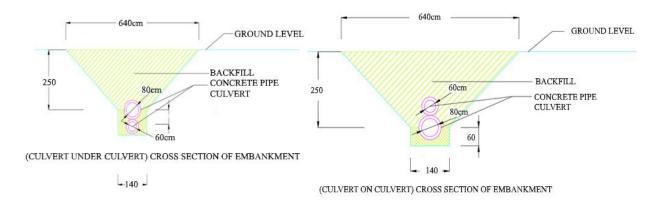
a) Culvert under culvert
