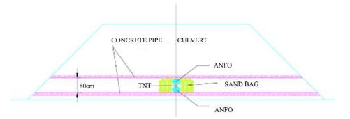
Figure 10. Cross-section image of the first test setup
