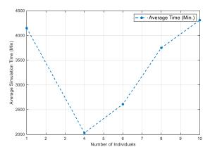
**Figure 12.** Completion time graph of the optimization process according to the number of individuals (1000 iterations)
