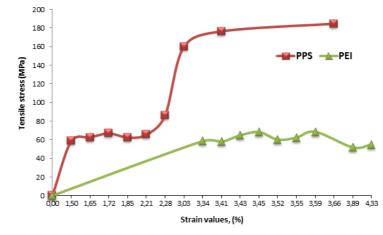
Figure 11. Tensile stress-strain curves for PPS and PEI
