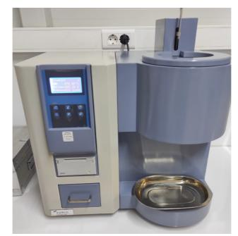
Figure 7. Melt flow index test of polymers
