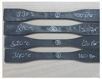
Figure 2. Tensile test specimens for PPS
