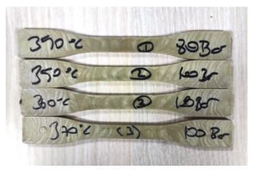
Figure 3. Tensile test specimens for PEI
